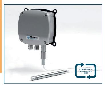
The WR283 relative humidity sensor uses the Hygrosmart module, integrated in the interchangeable probe and cable. This device can be used in high-temperature applications thanks to the remote placing of the measurement element and its small overall size. The interchangeable probe allows for simple re-calibration and lower maintenance costs.
