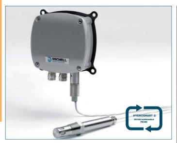
The WR285 relative humidity sensor uses the Hygrosmart module, integrated in the interchangeable probe. This device can be used in high-temperature applications due to the remote measurement element and its small overall size. The interchangeable probe allows for simple re-calibration and lower maintenance costs.
