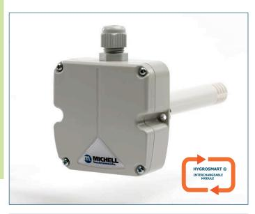
The DT269 transmitter has a I7000 Hygrosmart module. Thanks to this solution, the sensor can be changed on site quickly and simply, providing greatly reduced maintenance costs. The transmitter does not need re-calibration after the sensor is changed.
