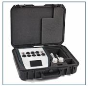
The HygroCal100 allows you to automate your calibration procedure with ease, and will provide a complete logged output of all probes under test against the reference instrument in csv format, ready to download to your USB memory device.
