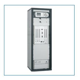
The DCS system is a complete rack-mounted calibration station capable of producing a flow of air (or nitrogen) at a pre-specified range of dew-point temperatures from a minimum of -100°C (-148°F) to a maximum of +20°C (+68°F). Through customization the DCS system can be PC controlled for automated calibration sequences or manually operated at pre-determined dew-point set points.
