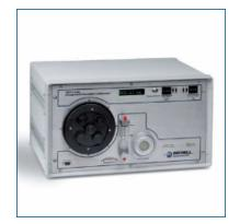
The OptiCal is a premium calibration solution for humidity sensors. The standalone and transportable humidity calibrator requires no external services other than mains power, and features an integrated chilled mirror reference instrument to enable the operator to perform calibrations that are traceable to national standards.
